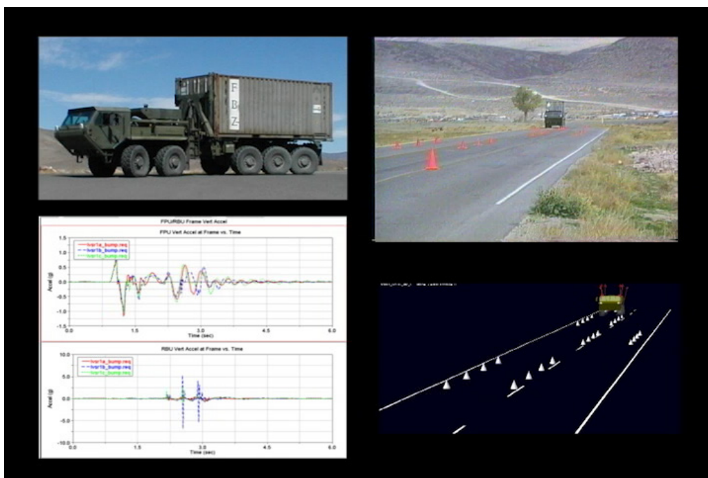
Figure E-5: Correlating Simulation and Test Results.
