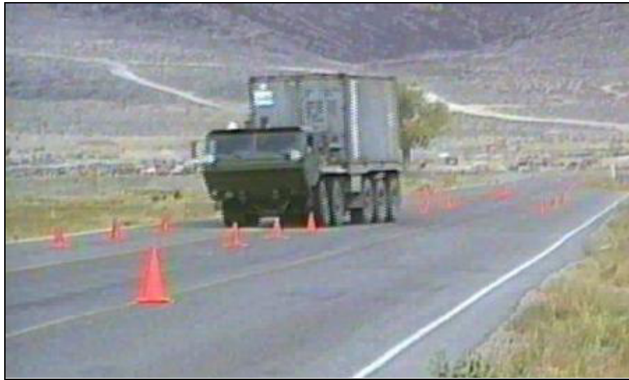
Figure F-3: LVSR-TD 10 x 10 Prototype During Double Lane Change Testing.
